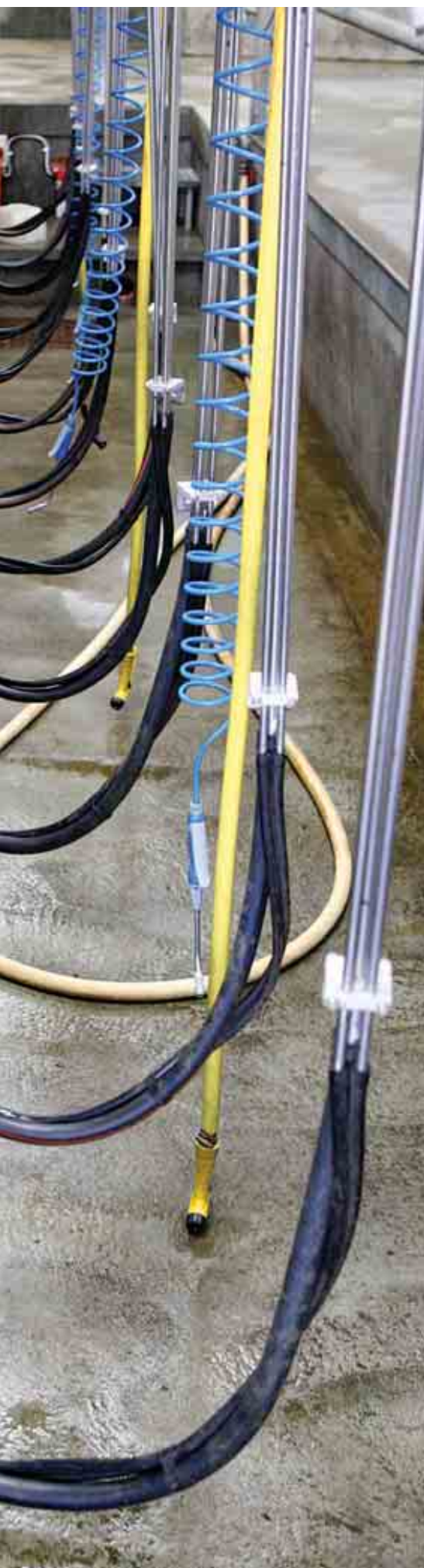
Flattening of the long milk tube at the milk entry to the milk line. Milking takes longer and cell counts can be adversely affected.
