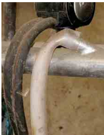
Flattening of the long milk tube at the milk entry to the milk line. Milking takes longer and cell counts can be adversely affected.
