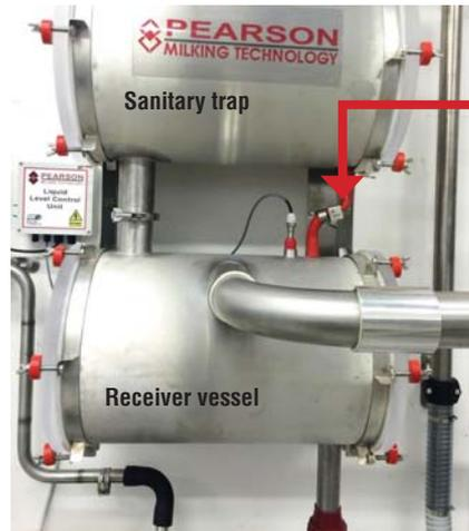
**The wash drain tube valve between the sanitary trap and the milk receiver must be closed during milking, otherwise drain-back, if any, will affect TBC.**
