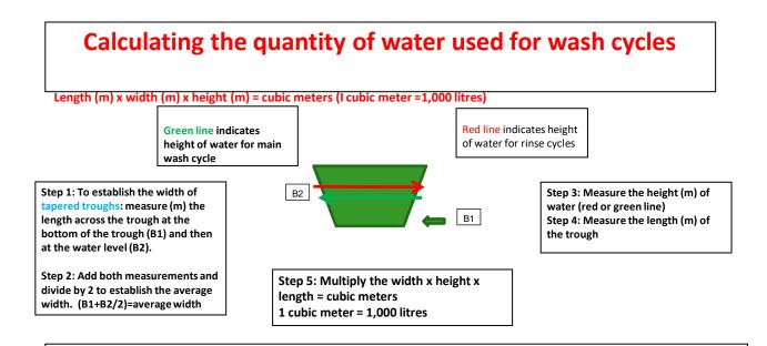
Target water levels for Rinse Cycles – 14 litres per milking unit Target water levels for the main wash cycle (hot or cold water) - 9 litres per milking unit
